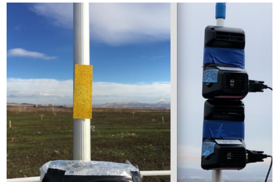
Water-sensitive paper (left) placed above real-time drift monitors (right) used in the orchard filed studies.
