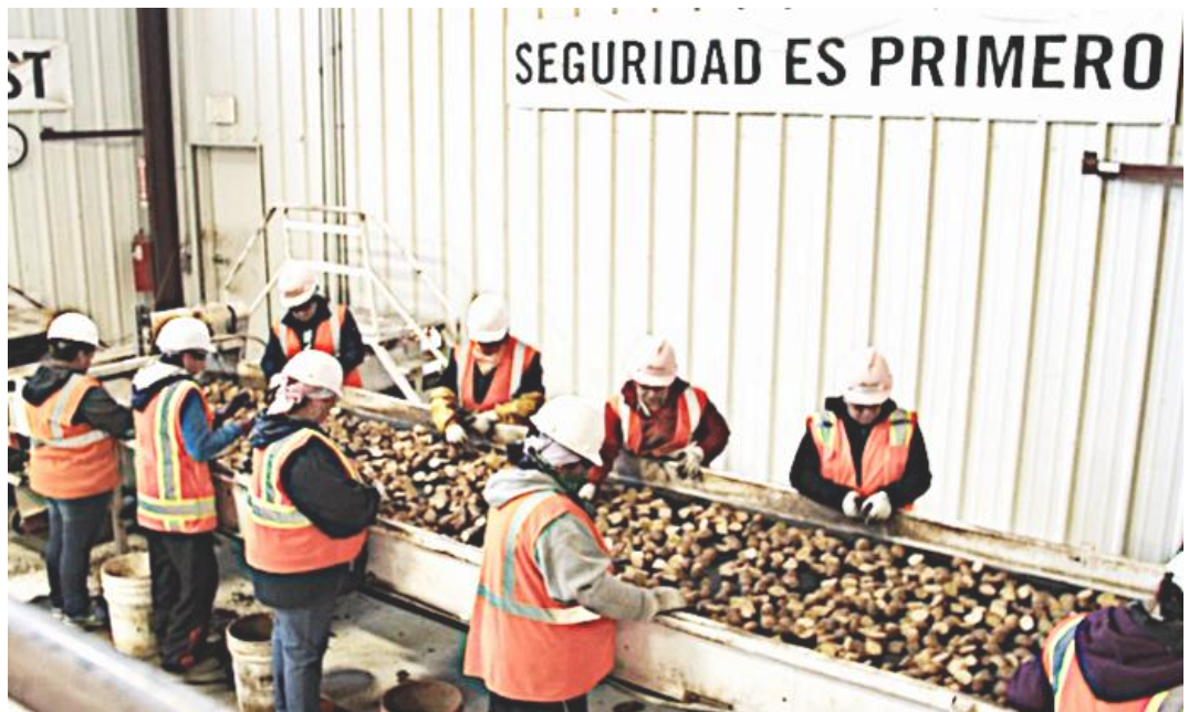
Cutting potato seed pieces is a task that can present injury hazards, as it requires extended standing time and repetitive motion. Photographer: Matthew Blua
