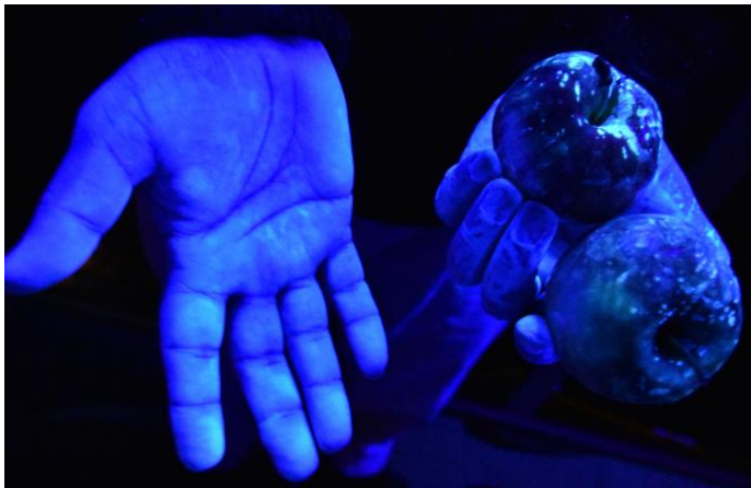
Fluorescent tracer (FT) glows under black light. PNASH uses FT to demonstrate pesticide contamination. Photo by Sarah Fish
